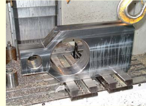
Contournage, surfacage, alésage, rainurage, perçage, taraudage
